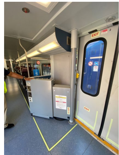
Figure 1. Alstom coach wheelchair lift
